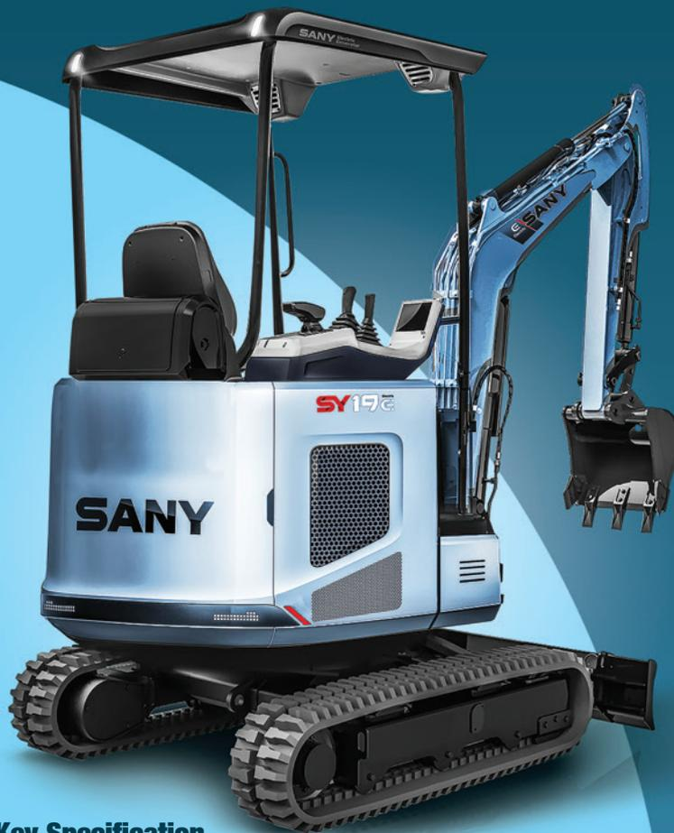
As well as **zero emissions** and considerably **lower noise** levels, the **compact electric SY19E** is equipped with a **lithium iron phosphate** (cobalt free) **battery** which allows for faster, safer and more efficient charging as well as a **significantly longer battery life** to reduce total cost of ownership.
